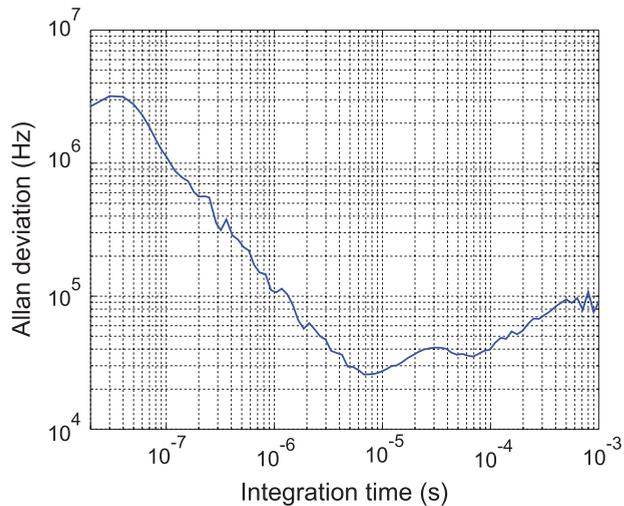
FIG. 4. (Color online) Allan deviation of beat measurements of the two independent and identically locked lasers with both electronic and optical feedback. The deviation has a minimum on the order of tens of kilohertz at the tens of microseconds time scale.
