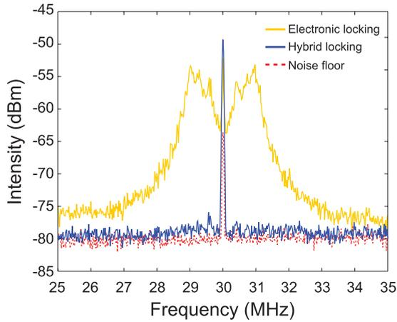
FIG. 2. (Color online) Spectrum of the signal on the locking detector which is modulated at 30 MHz. To obtain the locking signal, this is mixed down to dc. The curves indicate (i) optical feedback disabled (yellow/light curve), (ii) optical feedback enabled (blue/dark curve), and (iii) the detector noise floor (dotted red line), which is measured with the detector blocked. The resolution bandwidth was 30 kHz.
