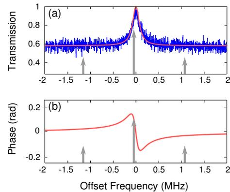
Fig. 2. The hole response. (a) shows the transmission of the spectral hole used, and (b) its corresponding phase shift. The arrows indicate the position of the carrier and sideband frequencies respectively.
