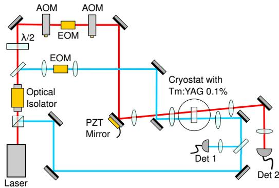
Fig. 1. The experimental setup. The experimental beam (in red) is frequency shifted and gated using two AOMs. The ultrasonic pulses were applied using a PZT-backed mirror. The beam is then steered through a prepared Tm:YAG 0.1%. The laser is locked to a spectral hole using a method similar to Bottger *et al.* [9] (path in blue), except with optical feedback.
